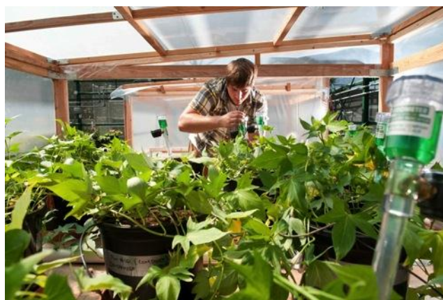
New growth chambers, custom built by Bill Hagopian (Jahren lab), are being used by Master's student Benjamin Czeck to test growth responses of sweet potato to rising carbon dioxide levels.
