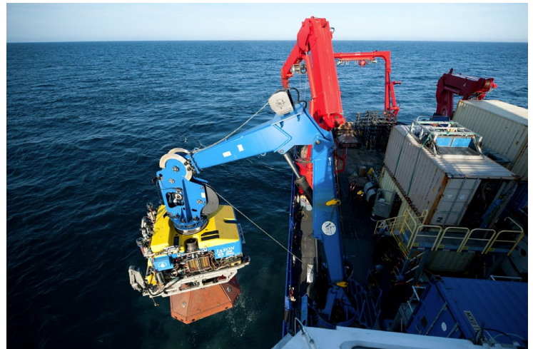
The ROV Jason being recovered onto the deck of the R/V Sikuliaq with an ocean bottom seismometer beneath it.
