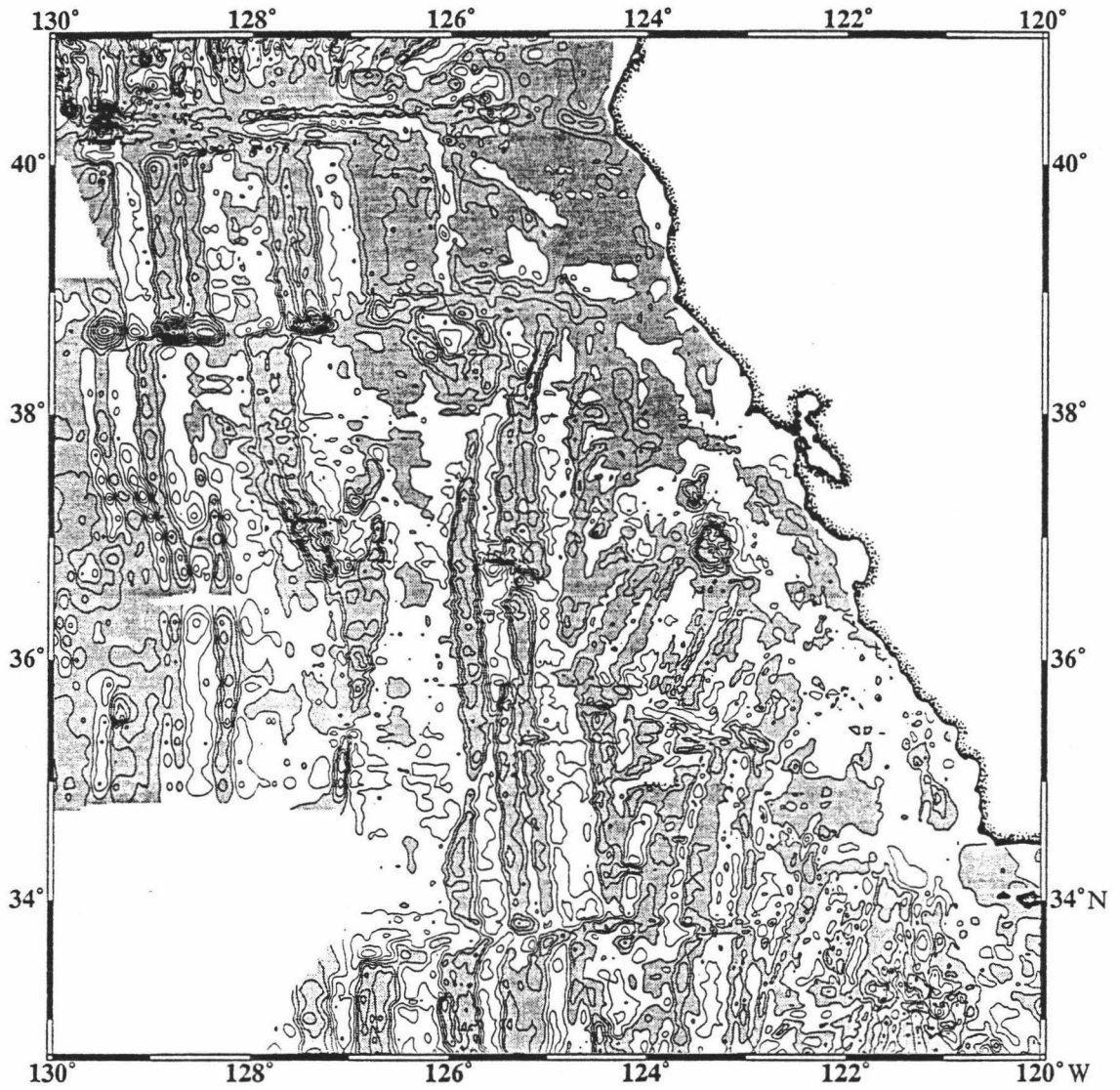
Fig. 9. Magnetic anomaly map of the entire data set gridded at 1 minute by 1 minute intervals. Contour interval is 100 nT. Positive anomalies (greater than -100 nT) are shaded.
