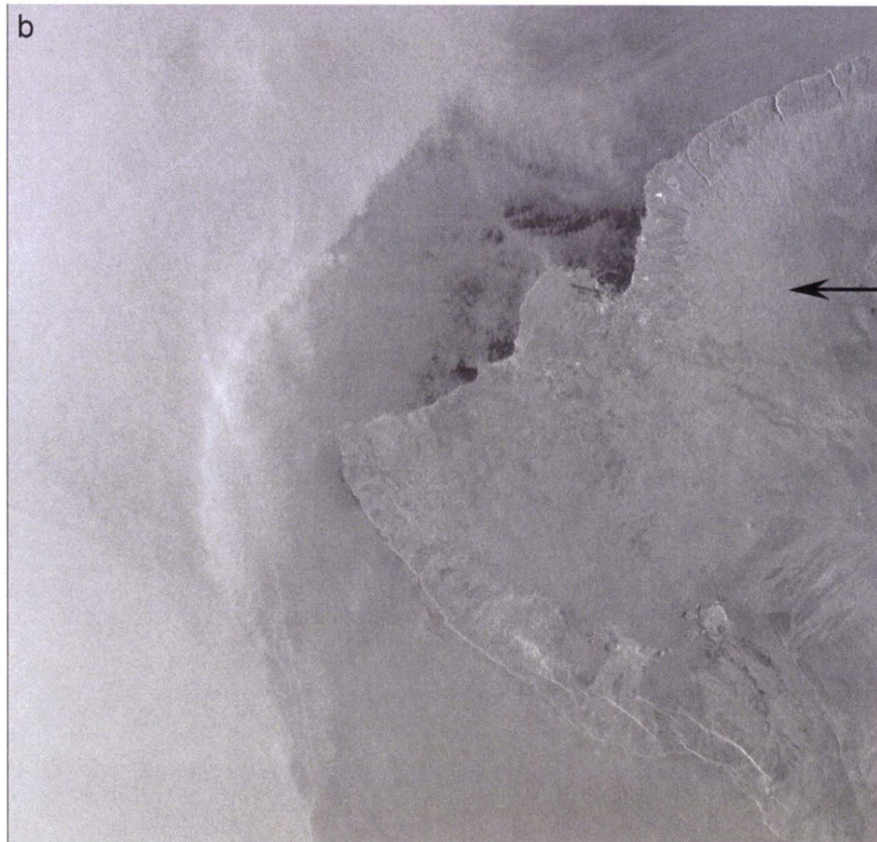
Figure 4: (a) Single-look raster image of the 20030212 single-look complex image (SLC) (MLR 1:1), (b) Multi-look intensity image (MLI) of the 20030212 SLC (MLR 1:5). Envisat ASAR IS2 track 429 frame 3213 (arrows indicate flight and look direction).
