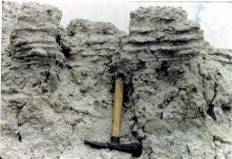
Figure 7. Photograph of layering (possible flow feature) in serpentine of UCC mine.
