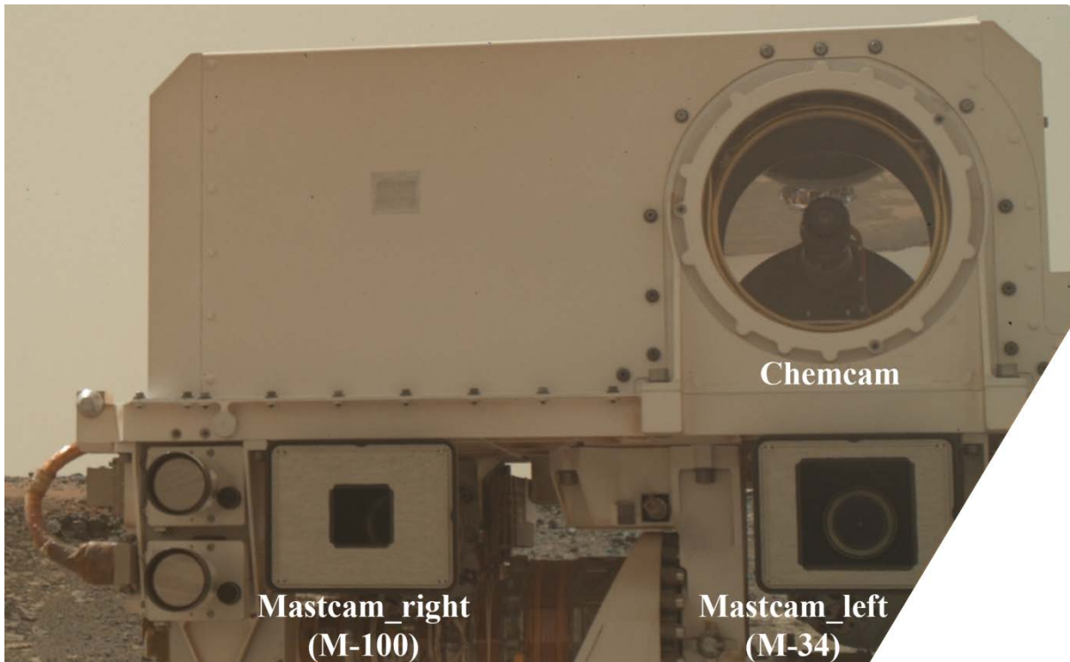
Figure 1.11: Portion of the latest MAHLI rover selfie, taken on sol 868, showing the Mastcam and ChemCam instruments. The ChemCam lens is 20 cm.
