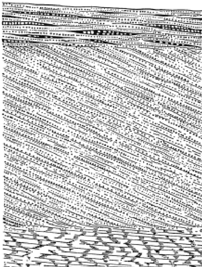
Figure 1.14: Geometry of deltaic deposits. (Figure 2 in Bhattacharya, 2006 after Gilbert, 1890).
