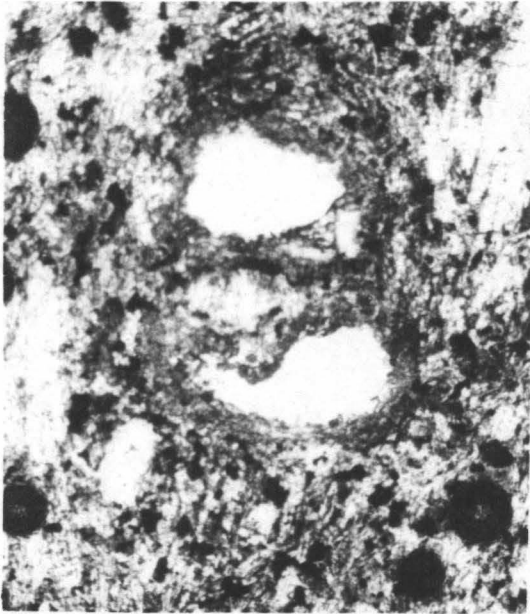
FIGURE 9: Photomicrograph of quartz grains with a pyroxene corona, sample R1238.8. The lower grain is 0.25 millimeters long.
