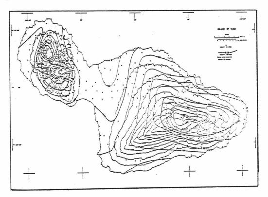
Figure 2. Complete Bouguer anomaly map of the island of Maui, Hawaii (Reproduced from Kinoshita and Okamura, 1965, p.34)
