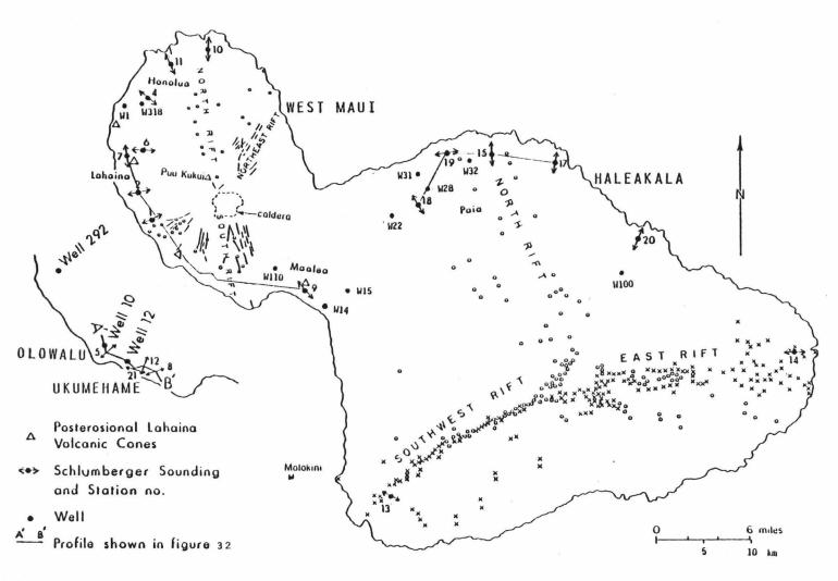
Figure 1. Map of Maui, showing principle volcanic rift zones, dikes (short lines), vents (circles and crosses), wells and Schlumberger sounding locations. (Modified from Macdonald and Abbott, 1970, p. 322 and 331).
