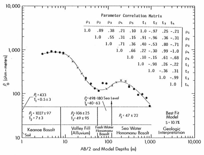
Figure 28. S20 apparent resistivity curve, best fit model and geologic interpretation.
