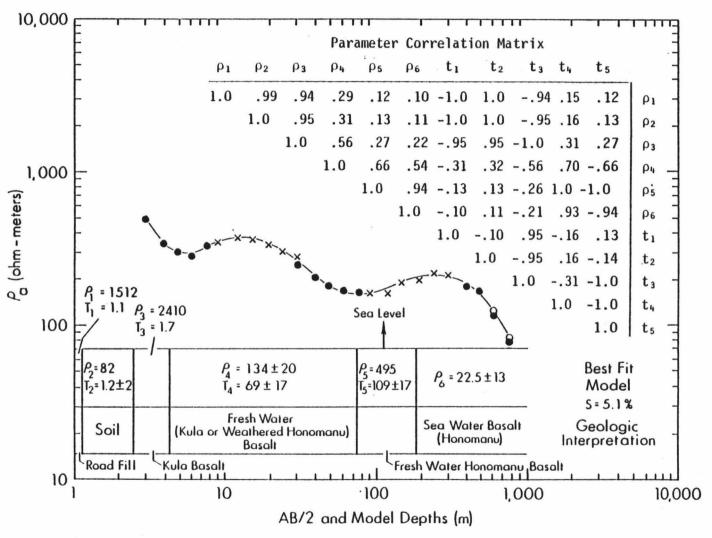
Figure 25. S17 apparent resistivity curve, best fit model and geolgic interpretation. Model parameters are unaffected by the coastal correction.
