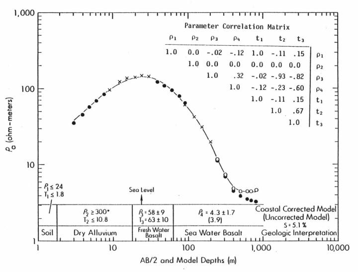
Figure 29. S21 apparent resistivity curve, best fit models and geologic interpretation. Note how application of the coastal correction flattens out the end of the curve.
