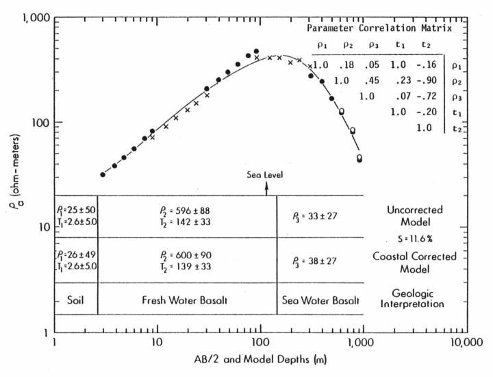
Figure 17. S7 apparent resistivity curve, best fit models and geologic interpretation.
