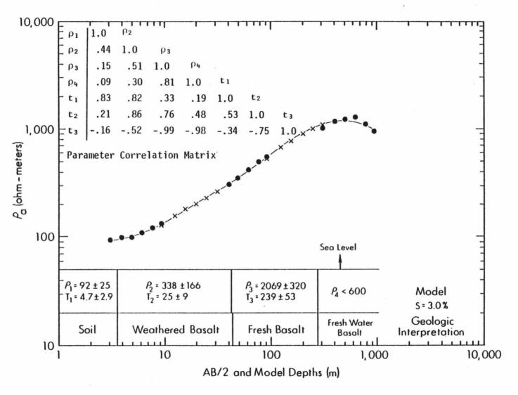
Figure 16. S6 apparent resistivity curve, best fit model and geologic interpretation.
