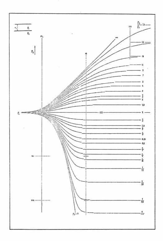
Figure 10. Two-layer master curves for the Schlumberger configuration. (reproduced from Compagnie Generale de Geophysique, 1955).
