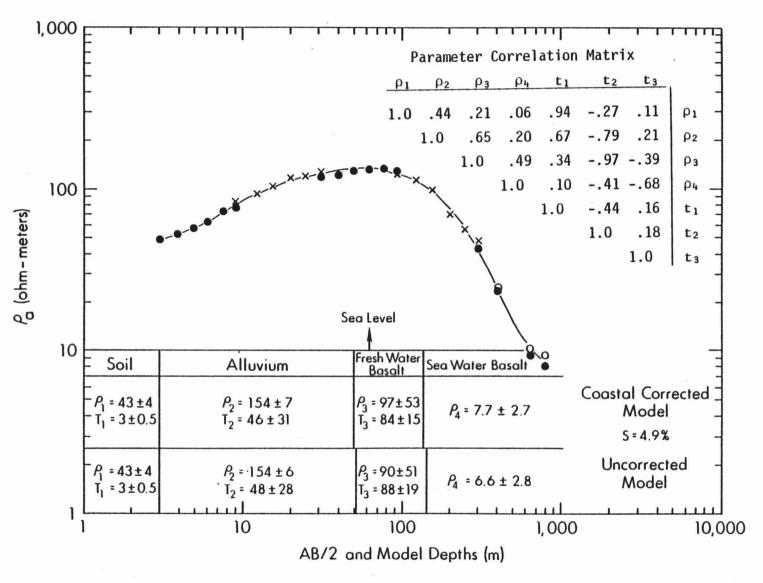
Figure 15. S5 apparent resistivity curve, best fit models and geologic interpretation.
