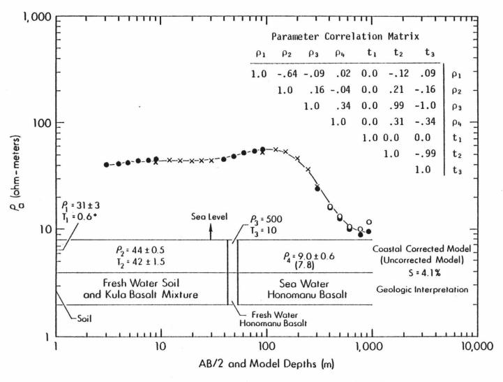
Figure 27. S19 apparent resitivity curve, best fit model and geologic interpretation.
