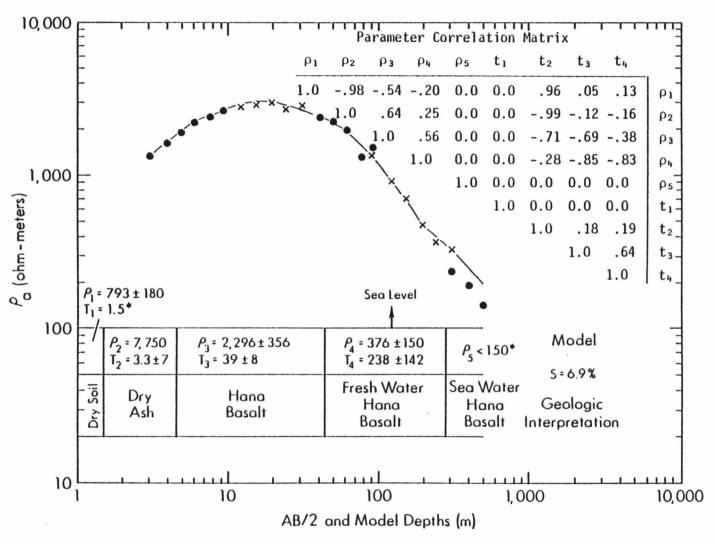
Figure 23. S14 apparent resistivity curve and geologic interpretation. The last 3 data points were shifted upward during the inversion.
