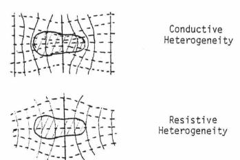
Figure 8. Distortion of potential lines at the earths surface due to local heterogeneities. Solid lines are equipotentials, dotted lines are current lines. (Modified from Kunetz, 1966, p.13).
