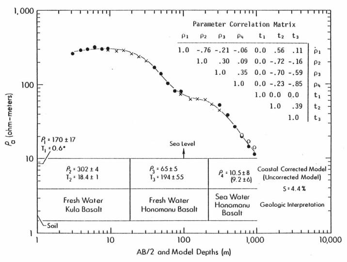
Figure 24. S15 apparent resistivity curve, best fit models and geologic interpretation.
