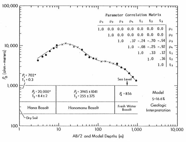
Figure 22. S13 apparent resistivity curve , best fit model and geologic interpretation, note high RMS error (S).
