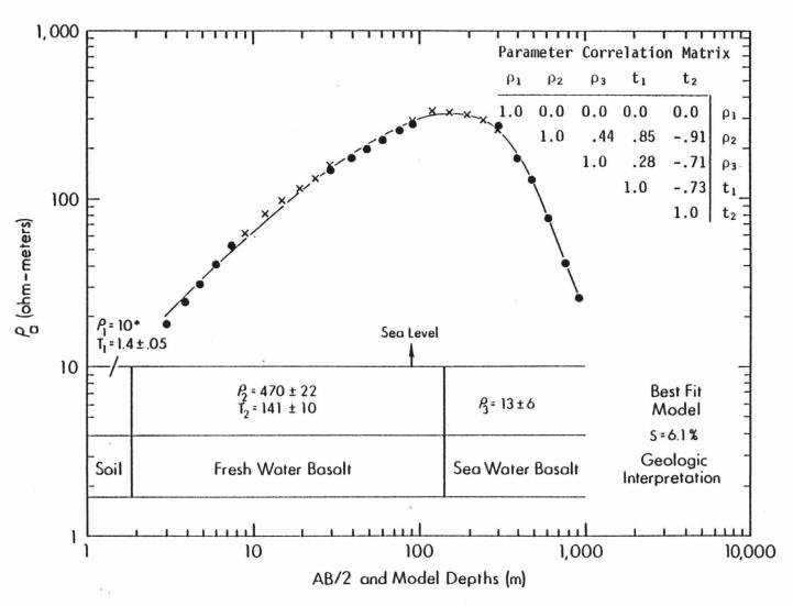
Figure 26. S18 apparent resistivity curve, best fit model and geologic interpretation.
