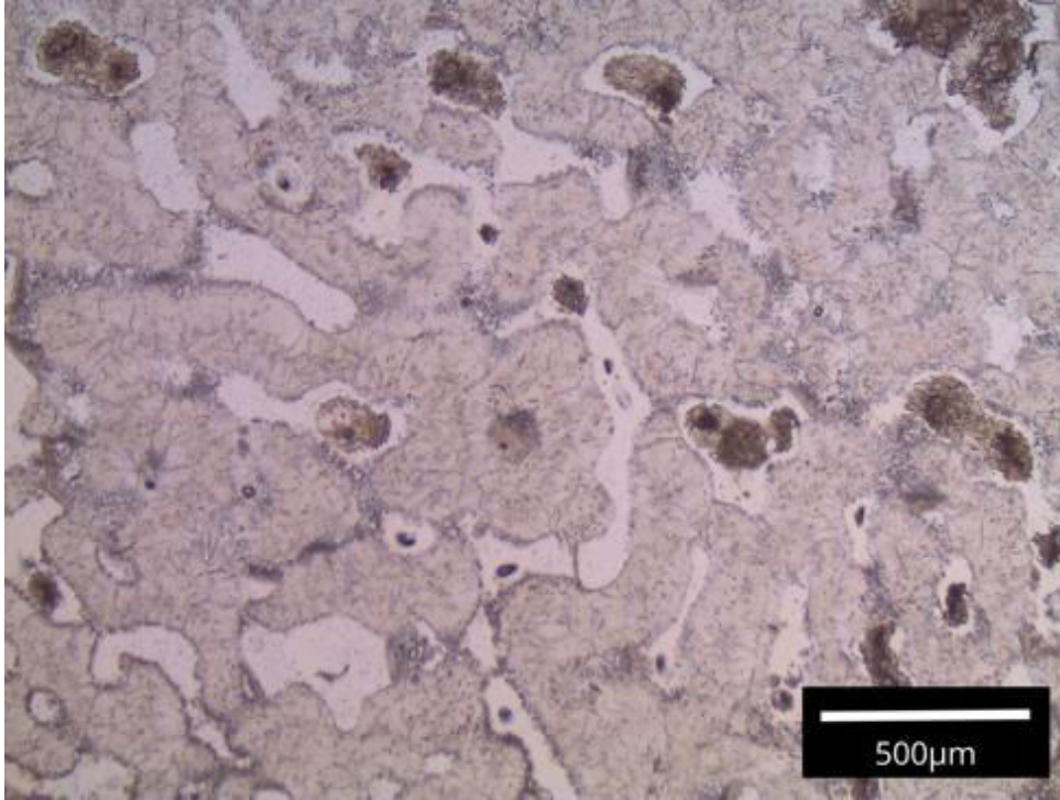
Figure 31. Plain Light Optical Microscope image of detrital material within pores of coral skeleton.
