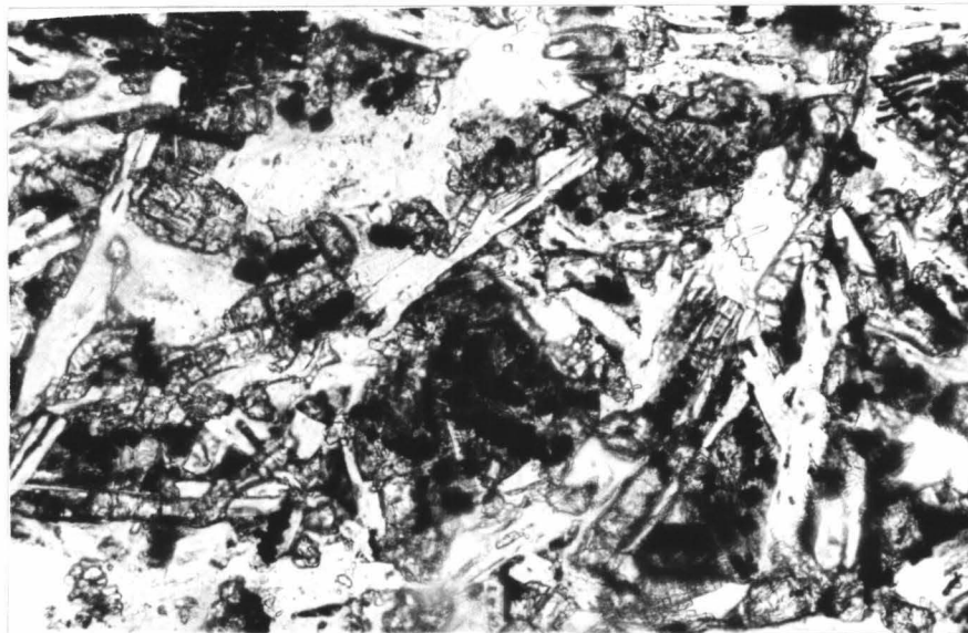
Figure 1. Dike groundmass of labradorite laths with intergranular clinopyroxene and included magnetite. Polars not crossed, X230.
